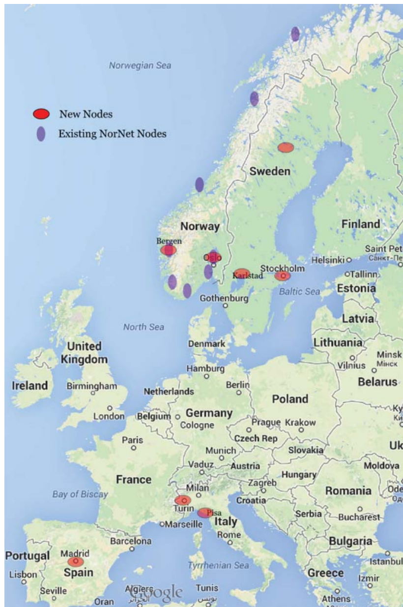
Figure 5.1 Geographical distribution of MONROE Nodes. MONROE builds on the existing NorNet Edge (NNE) infrastructure, consisting of 200 dedicated operational nodes spread across Norway.
