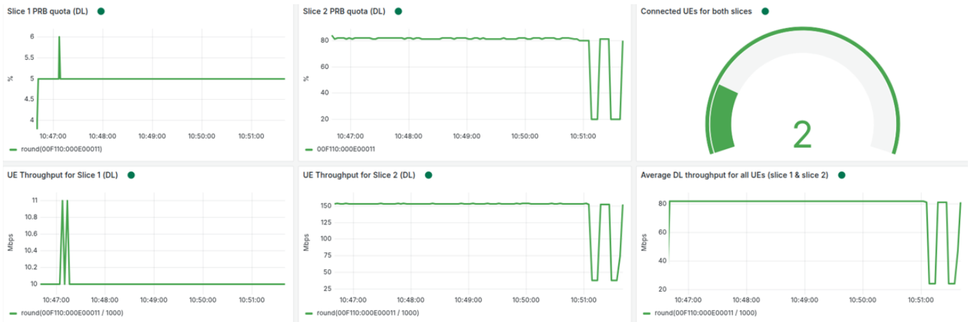
Fig. 5: Performance evaluation of the PIOR CM framework. The telemetry data (captured via Grafana) demonstrates the stability of Slice 2 PRB allocation (top center) and Throughput (bottom center) during the mitigation period (approx. 10:47:00 to 10:51:00), despite concurrent conflicting requests from the Throughput xApp.
