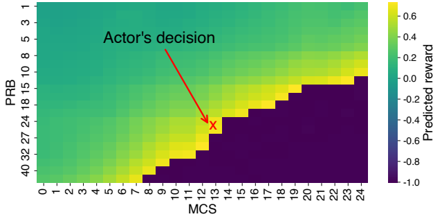
Fig. 13. Critic's reward prediction for SNR 20 dB and congestion factor \beta = .6 .
