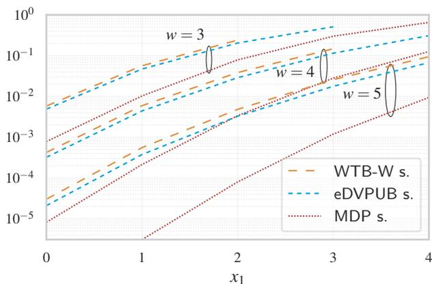
Fig. 14. DVP achieved by semi-static and dynamic schedulers for different backlogs  $x_1$  and deadlines  $w$ ,  $x_2 = 1$ ,  $N = 6$ ,  $p_e = 0.4$ .
