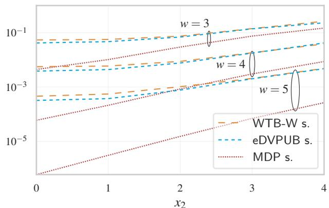
Fig. 15. DVP achieved by semi-static and dynamic schedulers for different backlogs  $x_2$  and deadlines  $w$ ,  $x_1 = 1$ ,  $N = 6$ ,  $p_e = 0.4$ .
