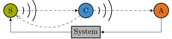
Fig. 1. Architecture of interactive applications with automated feedback. Sensor (S), controller (C), and actuator (A) operate in a closed loop via a two-hop wireless network path.
