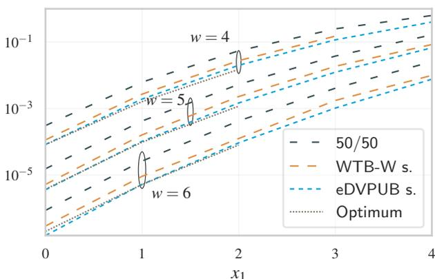
Fig. 6. DVP achieved by semi-static schedulers for different backlogs  $x_1$  and deadlines  $w$ ,  $x_2 = 1$ ,  $N = 4$ ,  $p_e = 0.2$ .
