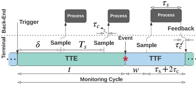
Fig. 1: Timing diagram of an arbitrary monitoring cycle.
